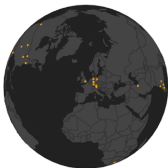
Figure 3: Use Case Example: Showing the geo position of users To implement this feature and additional transform step has been added that converts the Users IP-Address to an approximate Geo Information and adds this information to the the tracked event. This information is then queried using ElasticSearch .
